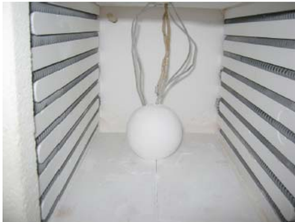
图 27 球形素坯内外温度测量示意图 [18] Figure 27 Diagram of thermocouple setting in alumina sphere [18]
